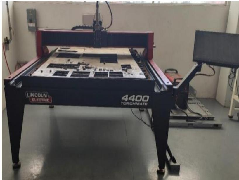
**Figura 14 .** Maquina de plasma LINCOLN ELECTRIC 4400.
