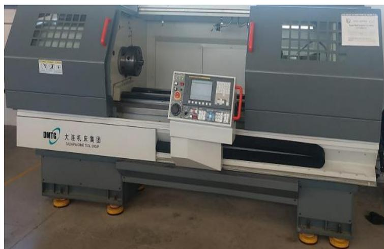
**Figura 15.** Torno CNC DMTG CKE 6150Z.
